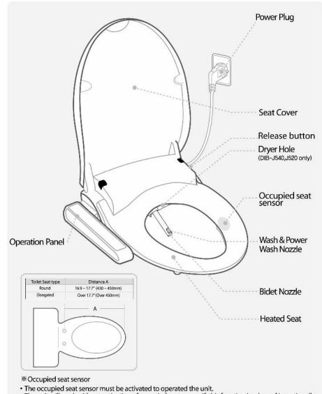
• The unit will work without activation of occupied seat sensor if this function is released intentionally.
